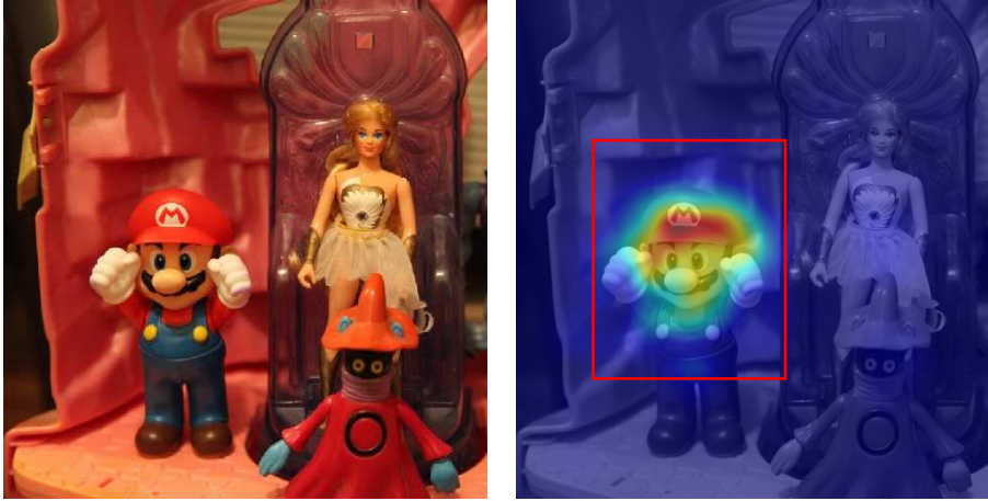
FIGURE 5.1 – The saliency map (right) computed for an input image (left) based on common-structure analysis on Instre dataset. Background clutter and objects not relevant for this dataset are automatically removed. The image is represented only by the region detected on the saliency map.
