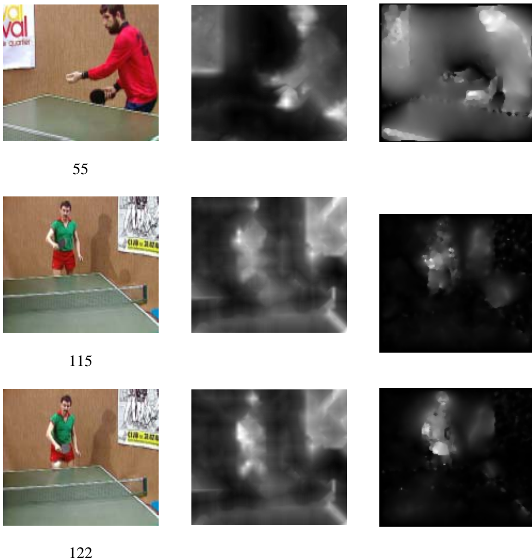
Figure 6 Results on the “table-tennis” sequence (numbers correspond to frames). Row-wise: original frame, saliency map and magnitude of the motion map
