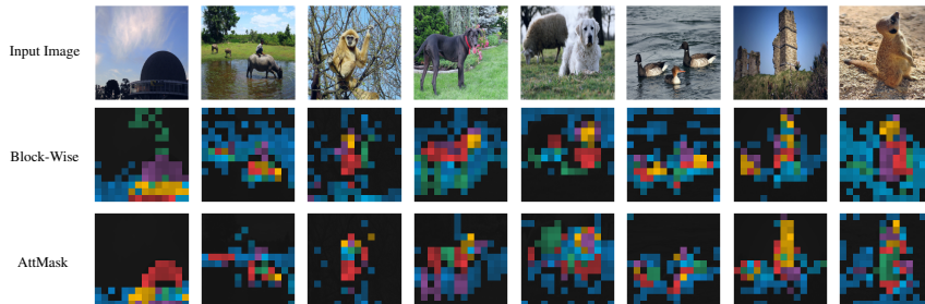
Fig. A5. Multi-head attention maps from the last layer, training iBOT with the default block-wise strategy from BEiT [2] and with our AttMask. From the attention matrix (5) of each head, we extract the attention map of the [CLS] token and display in different color per head the patch tokens that are included in the top 60% of the attention mass.
