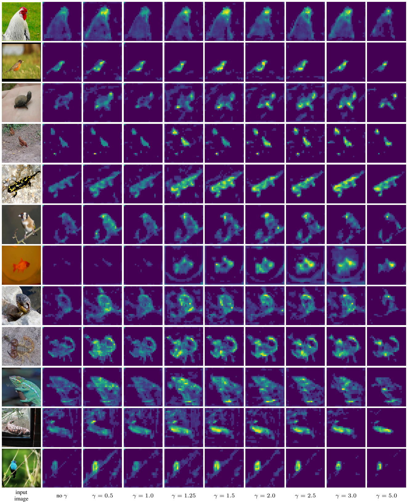
Figure C5. The effect of \gamma . Attention maps of ResNet-18 [31] with SimPool using different values of \gamma trained on ImageNet-20% for 100 epochs under supervision. We use the attention map \mathbf{a} (15). Input image resolution: 896 \times 896 ; output attention map: 28 \times 28 ; no \gamma : using the average pooling operation f_{-1} instead of f_{\alpha} (8). We set \gamma = 2 by default for convolutional networks.
