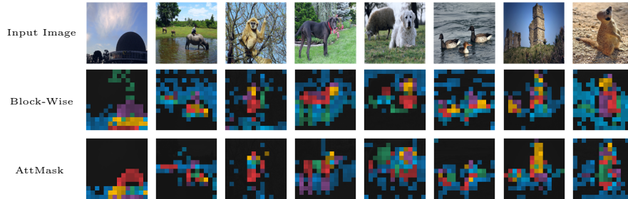
Fig. A1. Multi-head attention maps from the last layer, training iBOT with the default block-wise strategy from BEiT [1] and with our AttMask. From the attention matrix (5) of each head, we extract the attention map of the [CLS] token and display in different color per head the patch tokens that are included in the top 60% of the attention mass
